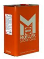
**APPLICATION:** For interior and exterior use on weather beaten, crumbly and worn-out sandstone and other soft, highly absorbent mineral surfaces. Surface treated with HMK® S741 remains 100% vapor permeable, UV resistant, and leaves a natural appearance. Not effective on marble and most limestone.
